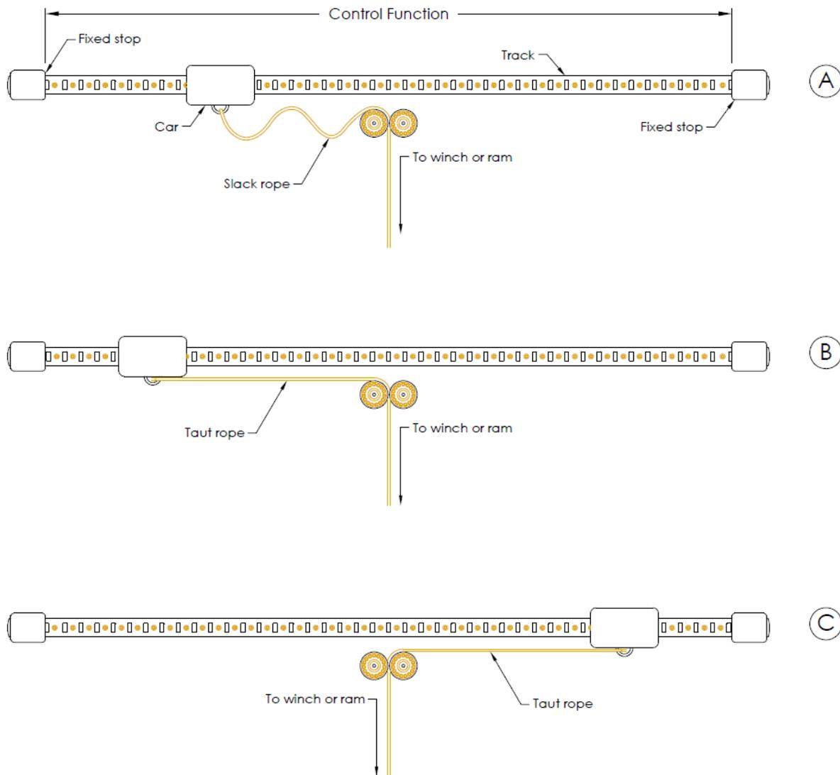
Figure 1 shows a **control system** in various configurations. A rope is connected to a car that can move on a track, where the position of the car maps directly to a **control function** of a **control surface**. The extension of the rope is adjusted by a winch or hydraulic cylinder. A typical example of such a system is a **mainsail traveller**.
